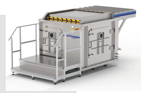
The IBF-1000R is designed for nanometer exact correction of rectangle optical surfaces up to 1000 x 1000mm. The plant is equipped with a high speed pumping system to minimize loading and unloading times.
