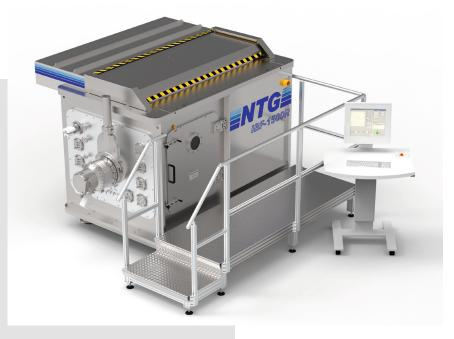
The IBF–1500R is designed for nanometer exact correction of rectangle optical surfaces (e.g. synchrotron mirrors). The plant is equipped with a high speed pump– ing system to minimize loading and unloading times.
