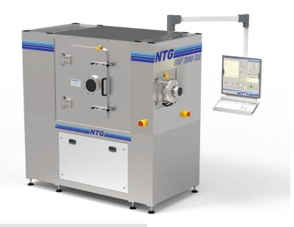
The IBF-200SE was launched in 2016 and is especially designed for industrial use. This new developed plant is for nanometer exact correction of small to medium sized optical surfaces.
