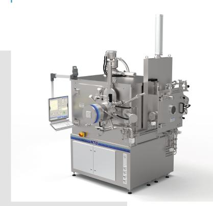
The IBF-350 RE is designed for form error correction on nanometer scale and additionally for inert gas ion beam etching as well as for reactive ion beam etching. Backside cooling, work piece heating, SIMS for end point detection, interface for clean room, beam monitoring with Faraday cup array and other helpful features are available. This plant is able to perform sub-aperture reactive gas ion beam etching.
