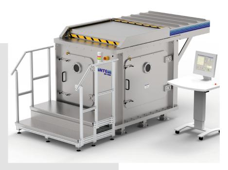
The IBF-700R is designed for nanometer exact correction of rectangle optical surfaces up to 700x700mm. The plant is equipped with a high speed pumping system to minimize loading and unloading times.
