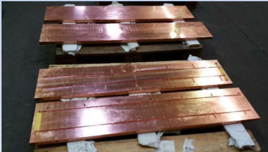
Electrode cooling channels
